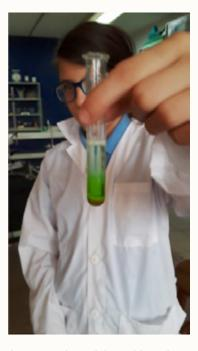
Testing for sugars, you place a small sample of food in a test tube and then add 3-4 drops of Benedict's solution. If sugar is present, the food sample will show green, yellow and brick-red depending on the amount of sugar. Yogurt tested positive for sugar. Showing the results of another test.
